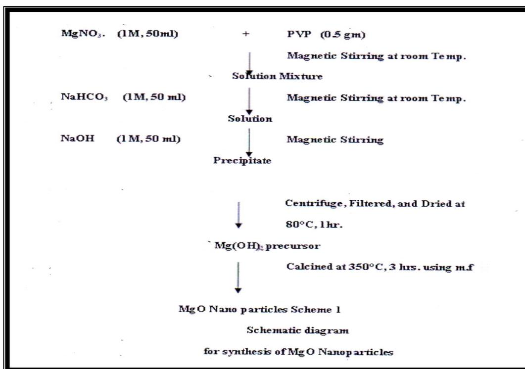
**Fig. 1 :** Stages of Manufactured Nano-MgO according to Ding *et al.* (2001)
