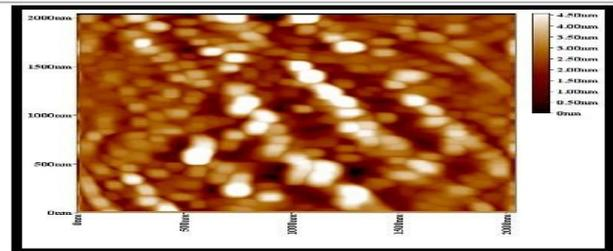
**Fig. 2 :** Size of Nano-MgO (locally manufactured) by Atomic Force Microscope (AFM) according to method by Ding *et al.* (2001)
